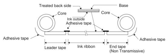
Fig. 2-9 Connection between leader tape and ribbon
